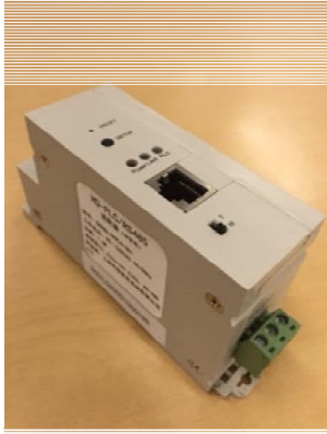
PLC / RS485 Converter (Shanghai PMS)
